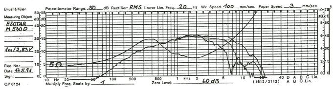
Frequency response and impedance curve of the ESOTAR® M-560 D on-axis, 30° and 60° (dist. 1 m).
