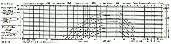
Levels of 1, 3, 10, 30, 100, 300 and 1,000 watts were applied while recording the curves. The parallel arrangement of the curves indicates that even fast 1,000 watt peaks do not produce any compression. Signal: Tone-Burst 10 ms, Signal-Pause 1:50.
